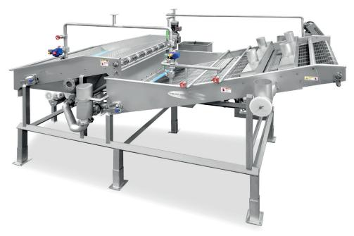
Two-Stage Potato Slice Washer shown with Air Sweep dewatering system.
