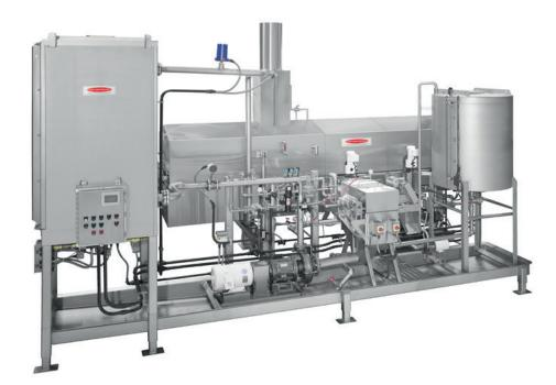
Pellet Poppers are available with a fryer support module (as shown) including the oil filter, pump, heat exchanger, storage tank and piping.
