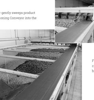
Filling stops automatically when the bin reaches capacity. The Bin Filling Auger levels product and begins filling the next preselected bin.
